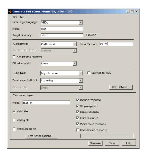
**Note** The Architecture pop-up menu also includes the new Distributed arithmetic (DA) option (see "Distributed Arithmetic Support for FIR Filters" on page 49).
